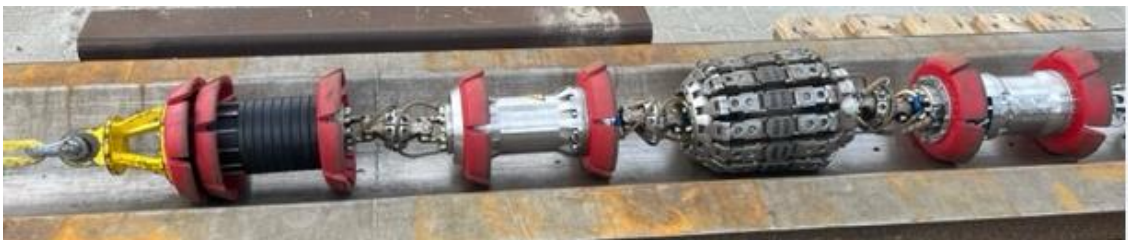
Figure 3: ROSEN standard 8" MFL-A tool with wear resistant steel brushes
