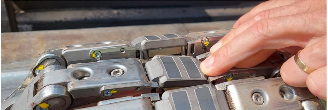
Figure 6: Flexible support of sensors and yoke
